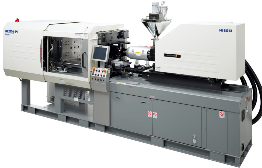
110T PIM Machine Made by Nissei Plastic Industrial
